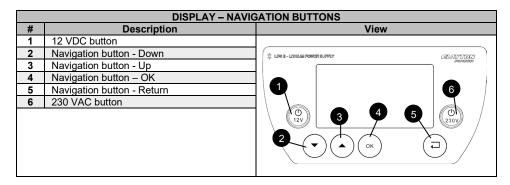
The 12 VDC and the 230 VAC buttons can switch the DC and AC output on and off. If both buttons are pressed and held for 10 seconds, the LPS II will reset without changing any settings.
