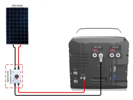
**WARNING:** Never exceed 50 Voc between DC Input minus and C2 from solar. Exceeding may cause damage to the unit.
