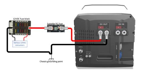
**WARNING:** Output fuse and cable size, including the grounding cable, should be rated according to the load being used.
