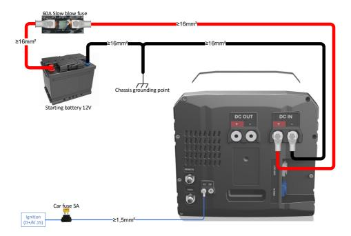
WARNING: Using the wrong cable size or a bad cable connection can cause overheating and a short circuit.
