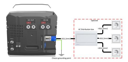
**WARNING:** A connection from the Neutrik 230 VAC Out connector to Chassis MUST be made for protective grounding.
