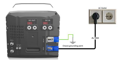
WARNING: 230 VAC will always be present on the AC output ports during AC charging.
