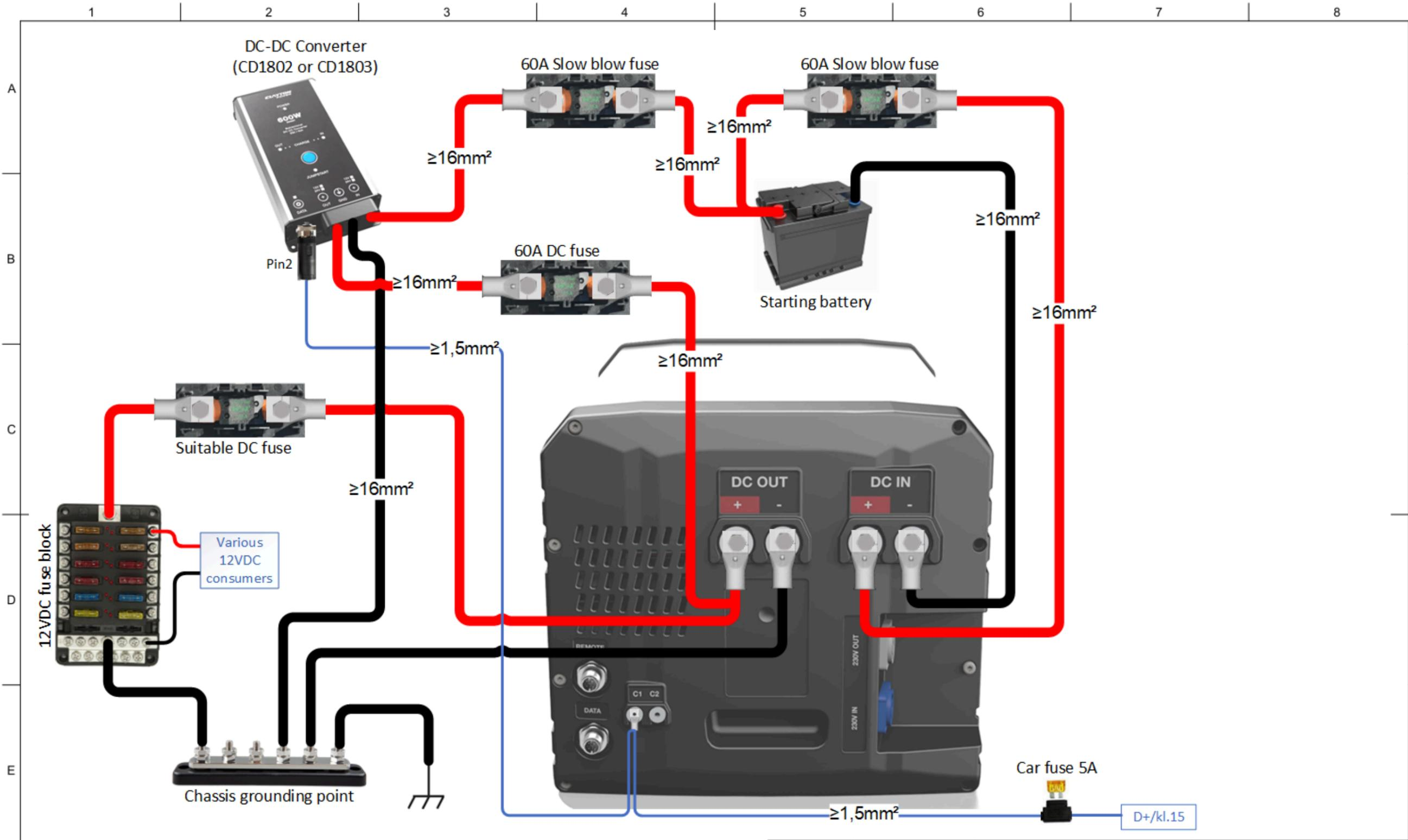
**Output fuse and cable diameter should be done to fit with the size of the load.**
