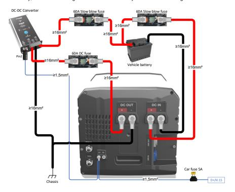
WARNING: Using the wrong cable size or a bad cable connection can cause overheating and a short circuit.
