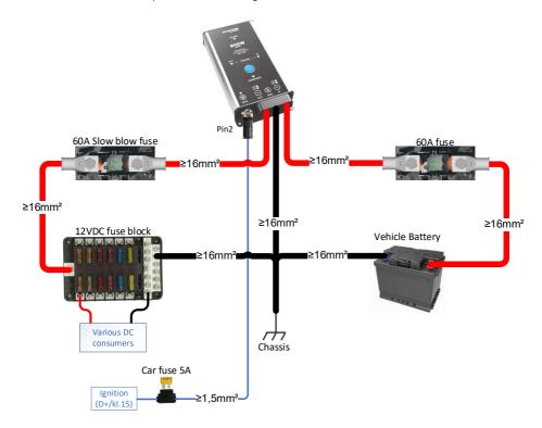
WARNING: Using the wrong cable size or a bad cable connection can cause overheating and a short circuit.
