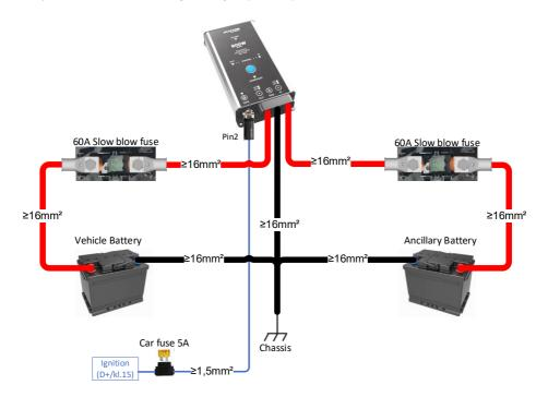
WARNING: Using the wrong cable size or a bad cable connection can cause overheating and a short circuit.
